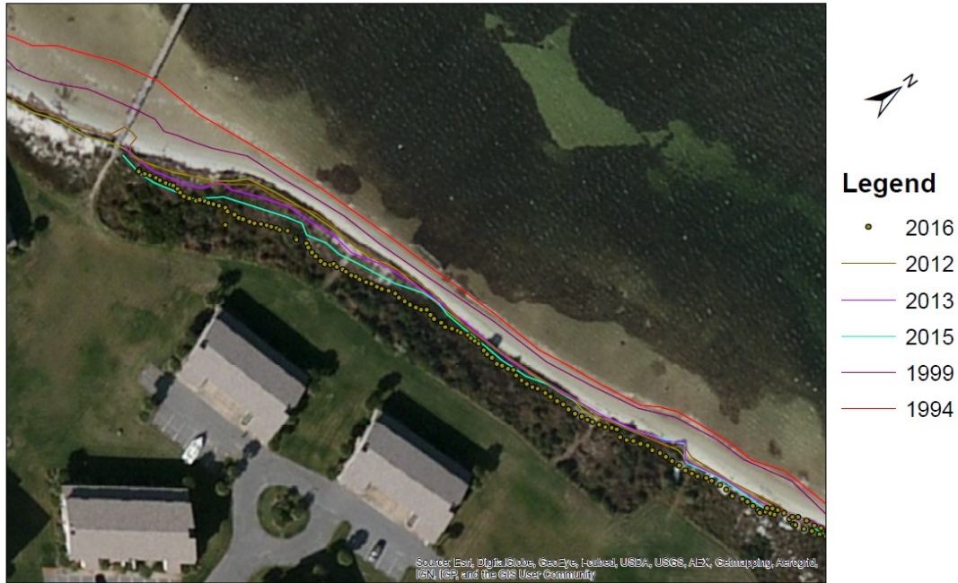
FIGURE 8: SHORELINE CHANGE FOR SECTION B IS EAST OF THE EXISTING DOCK FROM 1994- 2016
